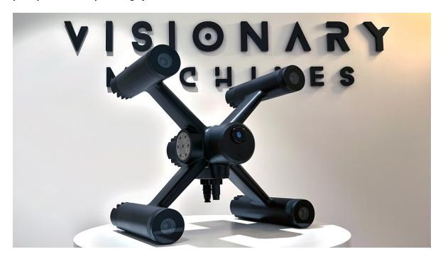
Visionary Machines, the Australian 3D spatial perception system company, has announced their 3rd generation Pandion™ sensor. The sensor enables machines to perceive the 3D world around them at long range, in real-time, in any lighting conditions, day or night.
